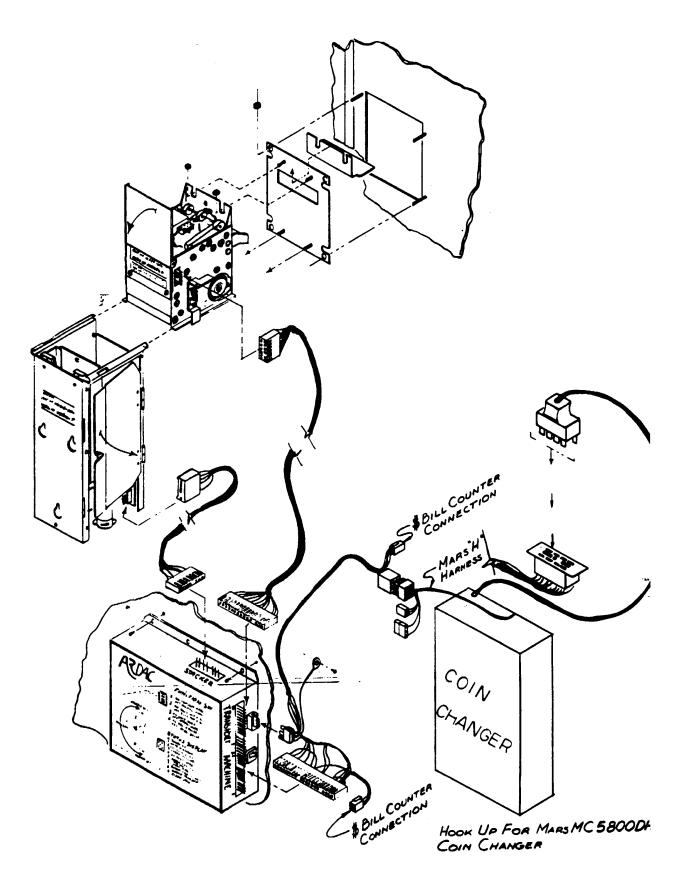
Component & Point to Point Wiring Harness Connections Blue Box System
