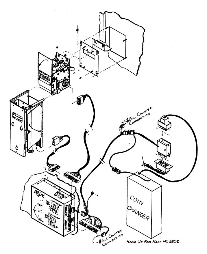
Component & Point to Point Wiring Harness Connections Blue Box System
